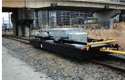
● Tractor-type track inspection system for conventional lines ●
