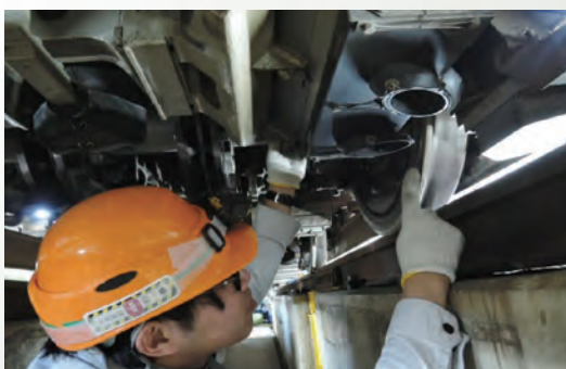
● Rail irregularity gauge inspection / Inspection car ●
